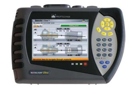
This add-on module runs on the ROTALIGN® Ultra platform and utilizes the unique 5-axis sensor to monitor continuously, in real-time and simultaneously both the vertical and horizontal parallel and angular displacement of rotating machinery, from cold to hot condition or vice versa and hence determining the relative positional change between coupled machines during operation. Running on the ROTALIGN<sup>®</sup> Ultra Shaft Expert platform, machine positional changes are monitored in real time
